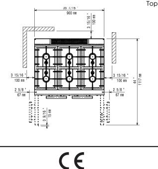
Modular Cooking Range Line 700XP 6-Burner Gas Range on Large Gas Oven
